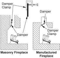
Figure 3 - Attaching Damper Clamp
